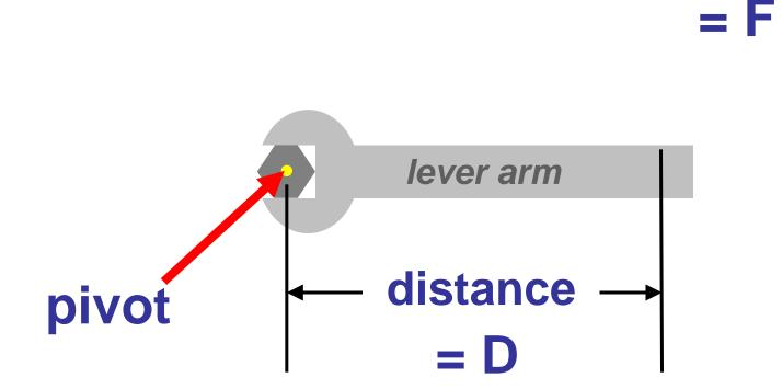
The distance must be <u>perpendicular</u> to the force.
