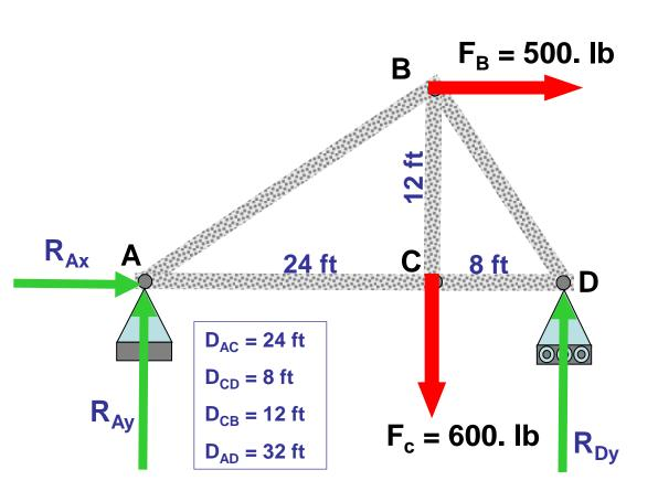
Replace the pinned and roller supports with reaction forces.
