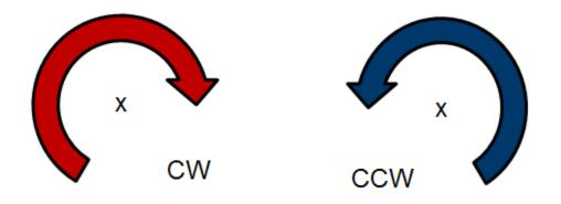
Drawn as an <u>arc</u> with an arrowhead acting about a point indicating direction of <u>CW</u> or <u>CCW</u>.
